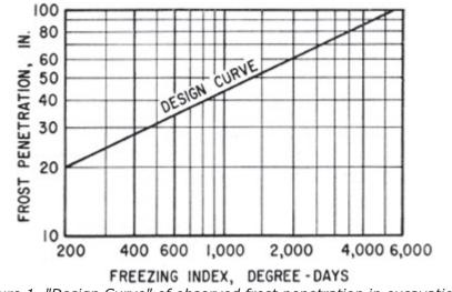
Figure 1. "Design Curve" of observed frost penetration in excavations.
